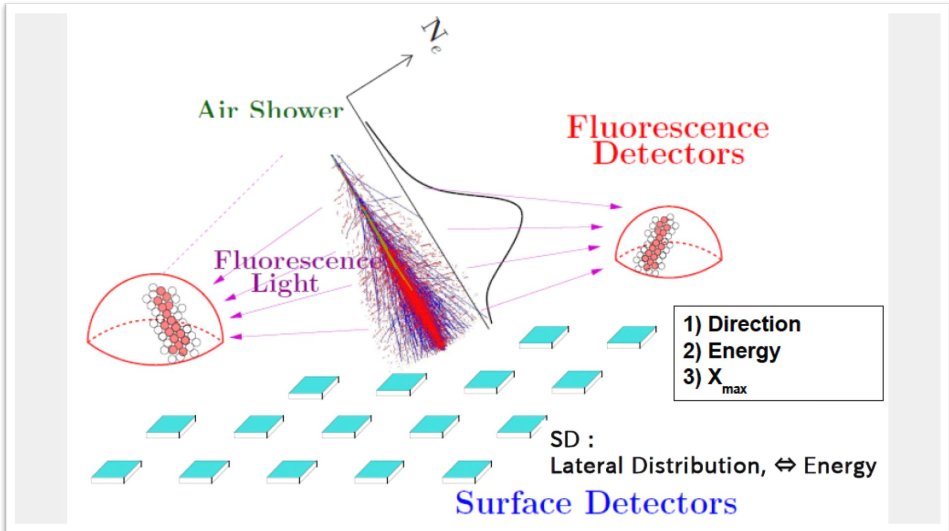
Surface detectors = single layer sampling calorimeter
